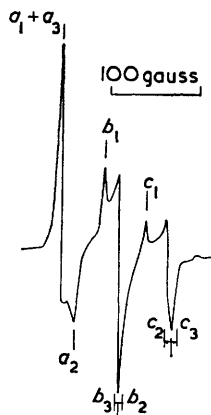
FIG. 2. Electron-spin resonance spectrum of NO 2 trapped in ice at 77°K. a_1b_1 = b_1c_1 = a_{yy} ; a_2b_2 = b_2c_2 = a_{xx} ; a_3b_3 = b_3c_3 = a_{zz} . g -Values measured at b_1, b_2, b_3 .
